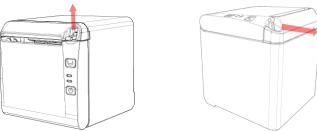
Fig. 4.4-1 Schematic drawing of paper roll installation/replacement
