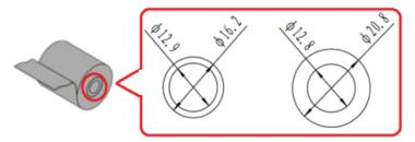
Fig. 4.5-3 core shaft of paper roll
