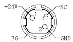
Fig.6.6-2 Schematic drawing of 24V power interface
