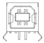
Fig. 6.2-1 USB interface connector
