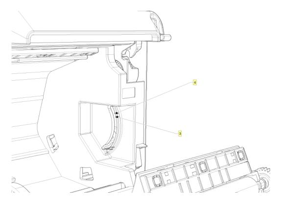
Fig. 4.5-2 Schematic drawing of paper near end position adjustment (output paper from the front)
