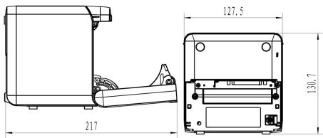
Fig.4.2-3 Printer maintenance and operation space
